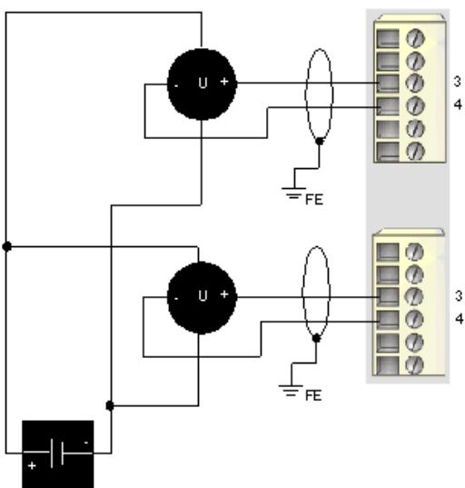
2 isolated analog actuators, external 24 VDC power supply
